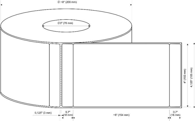
Roll, horizontal punched, thermo transfer, (ink ribbon) 200/76 mm roll size
