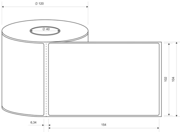
Roll, horizontal punched, thermo transfer, (ink ribbon) 120/40 mm roll size
